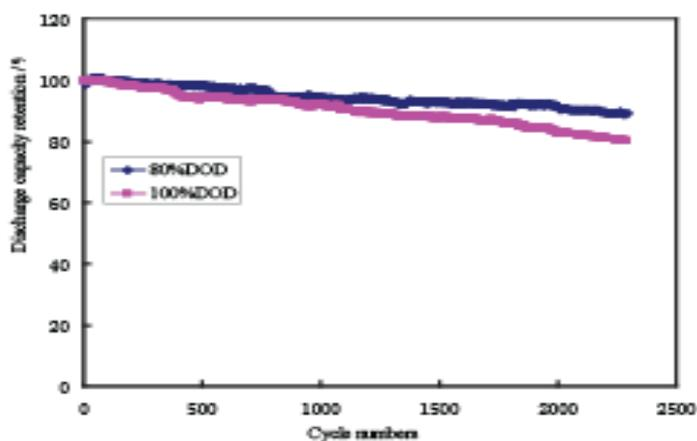
Drawing5 Lithium-ion power battery's different DOD cycle performance curve
