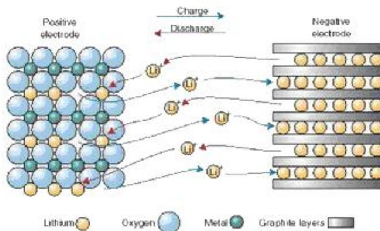
Drawing1 Lithium-ion power battery charge/discharge schematic diagram
