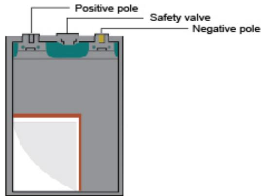
Drawing2 Lithium-ion power battery structure drawing
