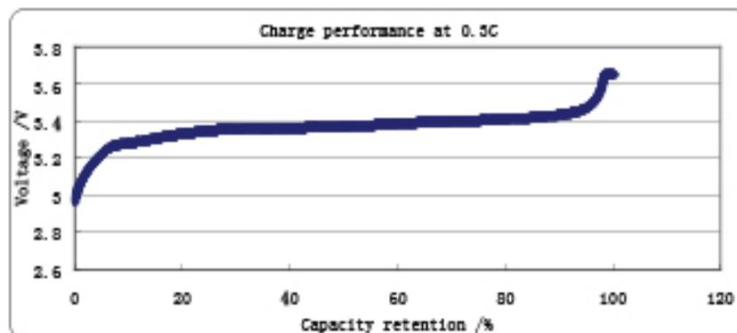
Drawing3 Lithium-ion power battery charge curve
