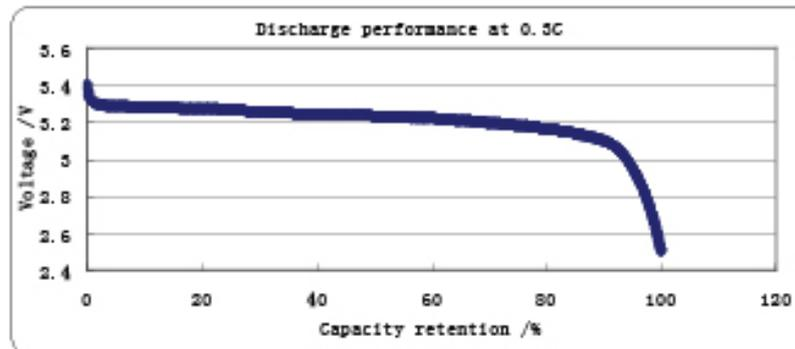
Drawing3 Lithium-ion power battery discharge curve
